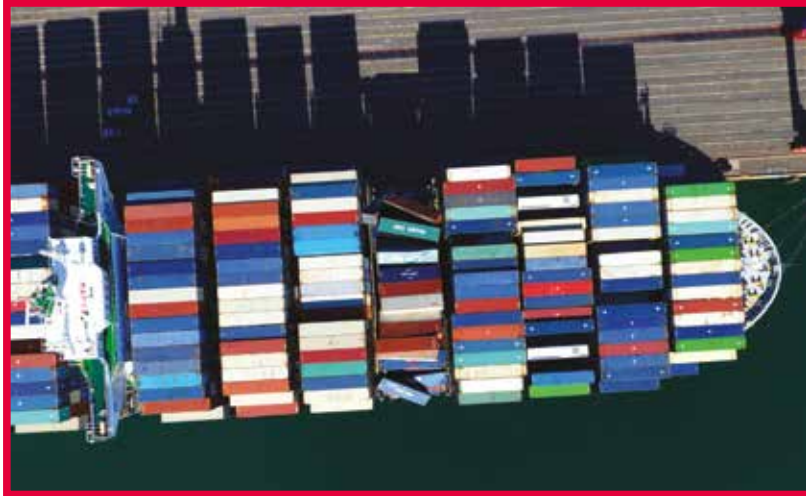
▲ The dangers of parametric rolling in severe conditions has recently been highlighted in a UK Marine Investigation Branch (MAIB) report on the collapse of three container bays and loss of 137 containers from the CMA CGM G. Washington Image: MAIB
