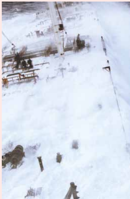
▲ The dangers of parametric rolling in severe conditions has recently been highlighted in a UK Marine Investigation Branch (MAIB) report on the collapse of three container bays and loss of 137 containers from the CMA CGM G. Washington Image: MAIB
