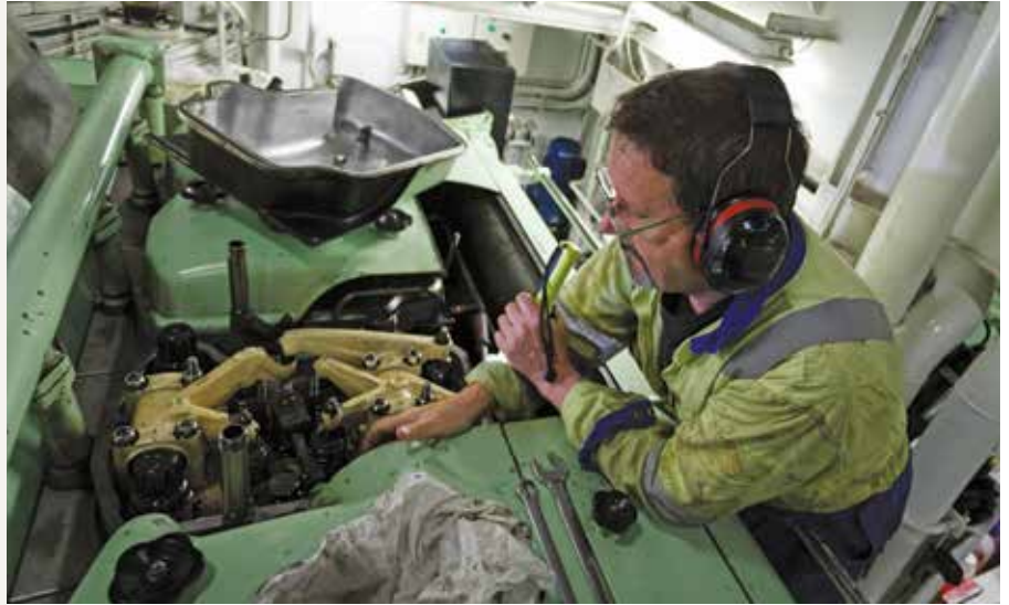
▲ The second engineer onboard an offshore oil platform supply vessel (PSV) in the North Sea, in the process of changing a fuel injector Image: Getty images/ DJDPhotographics
